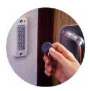
The AX100 access control kit is a compact, standalone single door controller supplied with Windows™ Plug and Play software for up to 4,000 cards - ideal for all doors, gates and barriers – in offices, factories, warehouses, hospitals, membership clubs etc.
