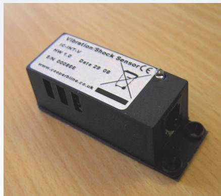
The vibration / shock sensor detects shock intensity caused by sudden knocks or hits and continuous vibration due to faulty ball-bearings on fans and other equipment.
