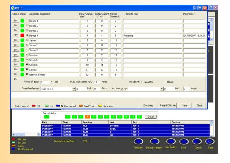
The main i-PDU sensor screen provides a clear overview of the current status of each i-PDU, a real-time graph is provided for instant visual analysis of the most recent transactions.
